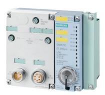
SIMATIC DP, CPU 1516PRO F-2 PN for ET 200pro, Central processing unit with work memory 1.5 MB for program and 5 MB for data, 1st interface: PROFINET IRT with 3-port switch, 2nd interface: PROFINET RT, 10 ns bit performance, degree of protection: IP65/67, SIMATIC Memory Card required, Connection module required
